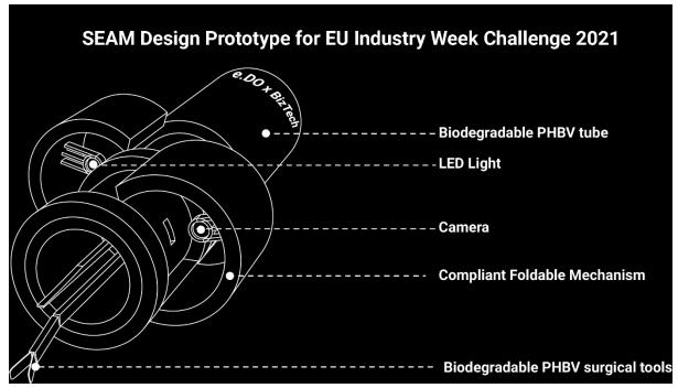
ESCP Team's **SEAM**: **S**urgical Instrument designed using the **e**.Do robot and **A**dditive **M**anufacturing
